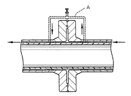
Figure 4 – Example of Monitoring Vent CRA Jumper
