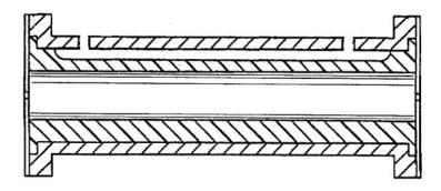
Figure 1 – Internally HDPE Lined Steel Pipe with Monitoring Vent Holes
