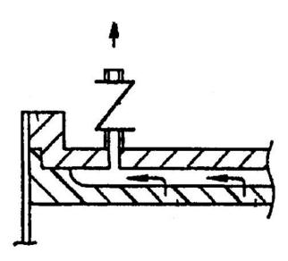
Figure 2 – Venting of Permeated Gas through Monitoring Vent
